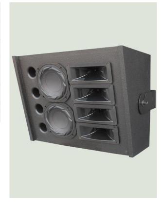
Because the directivity is very important (140° x 30° in this case), this new concept LAT series 2 way high tech surround speakers is based on Line Array technology and produces similar sound pressure levels (-3dB) frequency response in all seats of the cinema, be it in the central aisle, the side seats closer to the loudspeakers, rear and front ones.
