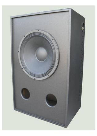
The classic highest quality system of the golden age of cinema business. THX Approved. 1x18" subwoofer system. This enclosure has many internal reinforces and vented gaps of 1,5 m. length with some parts in 30 mm. wood. This gives the best bass response you can imagine. The system is delivered assembled in one cartoon to save installations labor costs.
