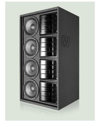
A Long Distance surround or proscenius surround high power system including with LAT2014 (Line Array Technology), which combines professional compression drivers with true isophasic horns to achieve an extreme -3dB coverage throughout the whole audience area. High power with Line Array Technology with 4 x 6" medium drivers plus 4 x 1" compression drivers + 4 x isophasic horns.
