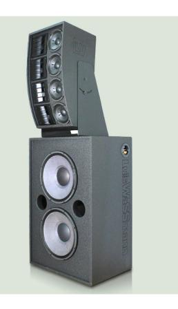
A screen system including LAT2014 (Line Array Technology), which combines professional compression drivers with true isophasic horns to achieve an extreme -3dB coverage throughout the whole audience area. 2 x 15" bass section plus a middle-treble section with Line Array Technology and 4 x 6" medium drivers plus 4 x 1" compression drivers + 4 x isophasic horns. For the biamp cut off frequency, please use our LW-8080 DSP Processor, which is delivered with all necessary
