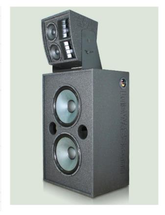
A screen system including LAT2014 (Line Array Technology), which combines professional compression drivers with true isophasic horns to achieve an extreme -3dB coverage throughout the whole audience area. 2 x 15" bass section plus a middle-treble section with Line Array Technology and 2 x 6" medium drivers plus 2 x 1" compression drivers + 2 x isophasic horns. We strongly recommend this model as the natural replacement to our discontinued products LW 2203-BI and LW 5107-BI.
