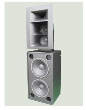
With the digital cinema in mind, we introduce our STATE-OF-THE-ART very high quality 4 way system for tri-amp, with built in network for mid-high/high. 2x18" bass loudspeakers + 2x10" midrange loudspeakers + the new coaxial driver 1x3,5" mid-high + 1,75" high driver. Evolution of our superb 5009, the LW 5109 improves the bass response with a new enclosure.
