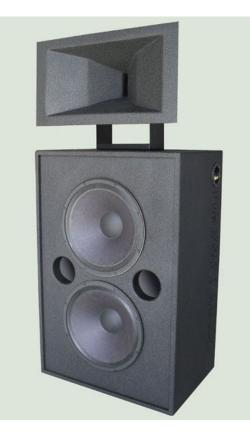
Evolution of our well known LW 3003, with a polyester 90° x 40° big horn for acoustic walls. It is now fitted with our SCD (screen compensation device) and our "Virtual Three Way Tech", thus eliminating the "comb filter" between both of the 15" bass units.
